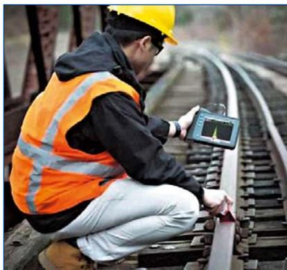
*The service includes the drafting of control procedures and the execution of non-destructive tests with surface methods (VT, MT and PT) and volumetric testing (RT and UT) performed by qualified Level II and III Operators according to UNI EN ISO 9712*
